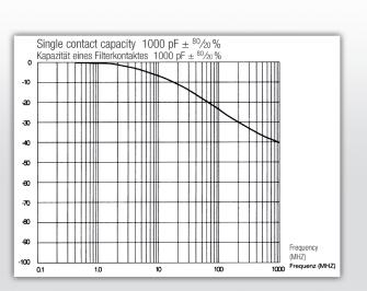
D-Sub filter connectors suppress interference of the input signals at the D-Sub device interface. PROVERTHA offers the range of filter connectors with filter capacitors for the suppression of crosstalk and harmonics, which act as low-pass filters. The cost-effective solution for the suppression of disturbances
