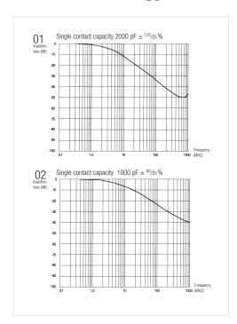
D-Sub filter connectors suppress interferences of the input signals at the D-Sub device interface via filter capacitors or as ferrite-equipped connectors
