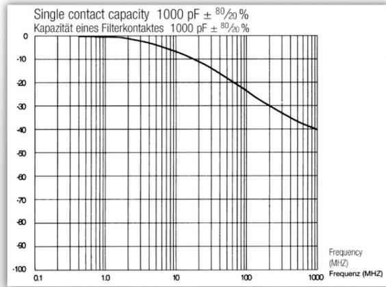
D-Sub filter connectors suppress interference of the input signals at the D-Sub device interface. PROVERTHA offers the range of filter connectors with filter capacitors for the suppression of crosstalk and harmonics, which act as low-pass filters. The cost-effective solution for the suppression of disturbances at high frequencies with lower attenuation requirements, the series of ferrite-equipped filter connectors.
