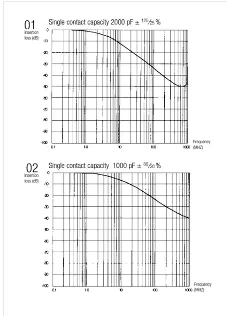
D-Sub filter connectors suppress interferences of the input signals at the D-Sub device interface via filter capacitors or as ferrite-equipped connectors
