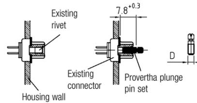
Variant B: Attachment set for existing connector with thread on solder side
