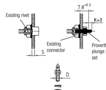
Variant C: Attachment set for existing connector with through hole
