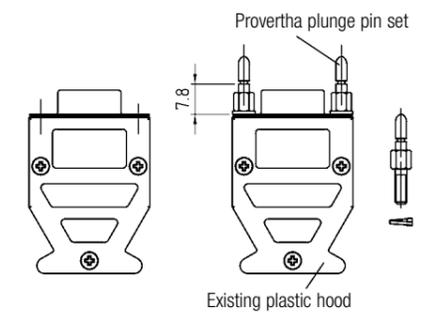
Variant E: Attachment set for connection hood-hood directly through housing wall
